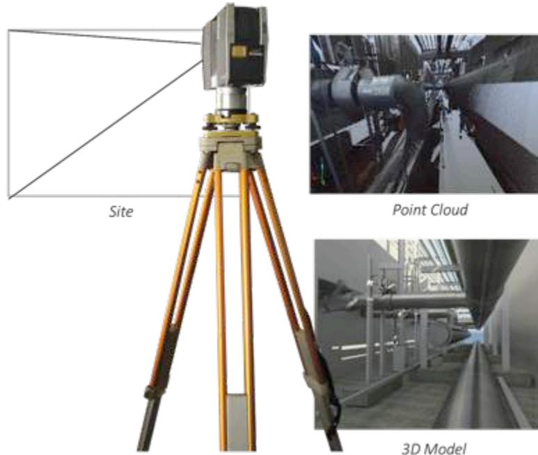
Capture and Extract highly accurate data points (+/-3mm) to point cloud
